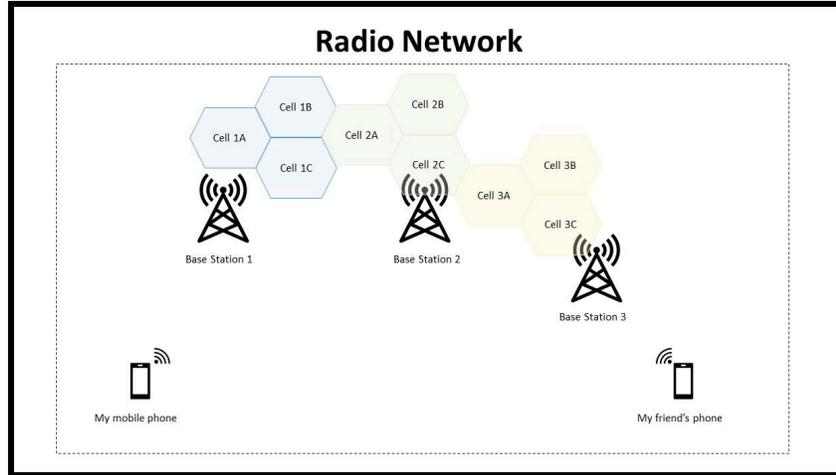
**Fig 10: Graphic illustration of a cellular network**
