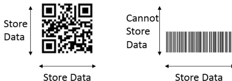
Figure 5: QR code can store data on vertical direction whilst barcodes cannot
